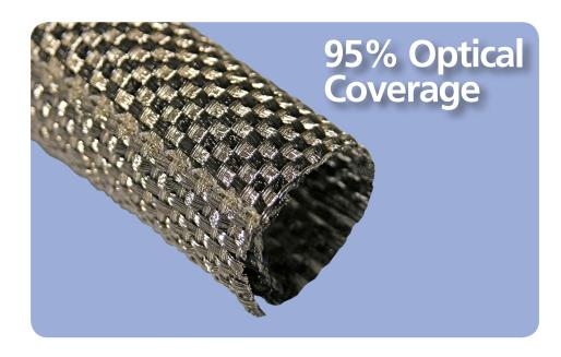
**ROUNDIT® EMI FMJ (Full Metal Jacket)** is a wrap-around sleeving designed for high performance EMI shielding of wire and cable bundles. ROUNDIT EMI FMJ is manufactured from PPS monofilaments and nickel plated copper.
